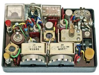
Internal view of the Neptun II transmitter. Note the miniature Morse key located in the right hand bottom corner.
